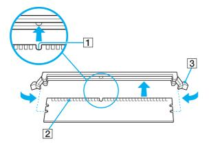
To avoid damaging a memory module or the memory module slot, move the side latches slightly outward to relieve pressure.
